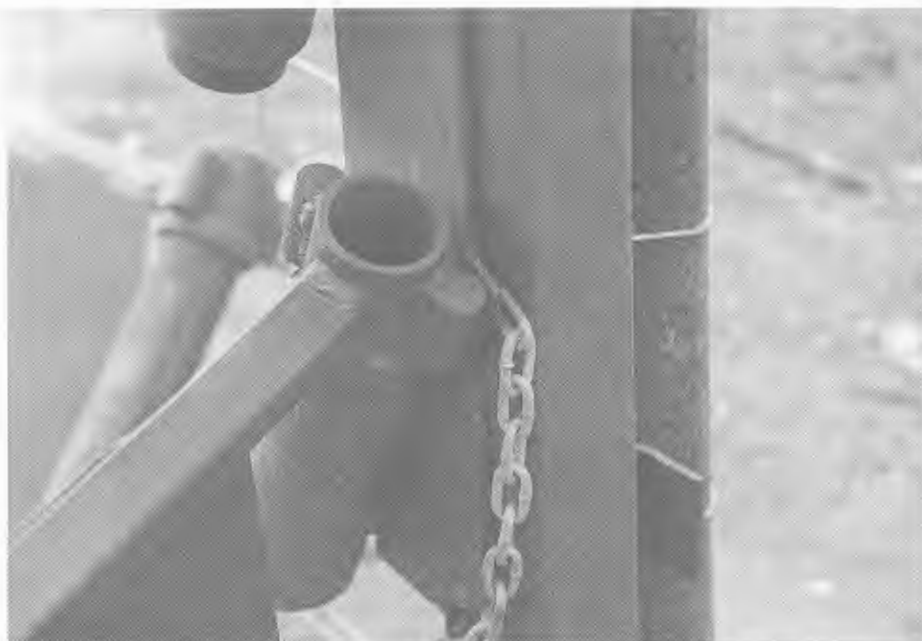
Collar fitted to sheep spear arm
