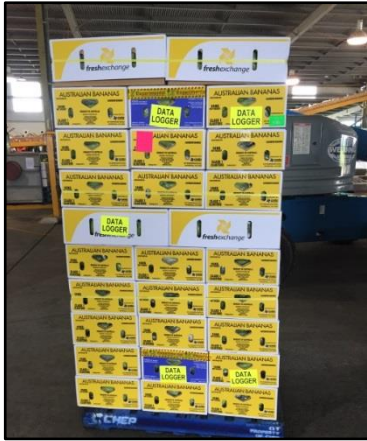
Figure 1. Data loggers placed at the top, middle and bottom of a pallet prior to despatch.
