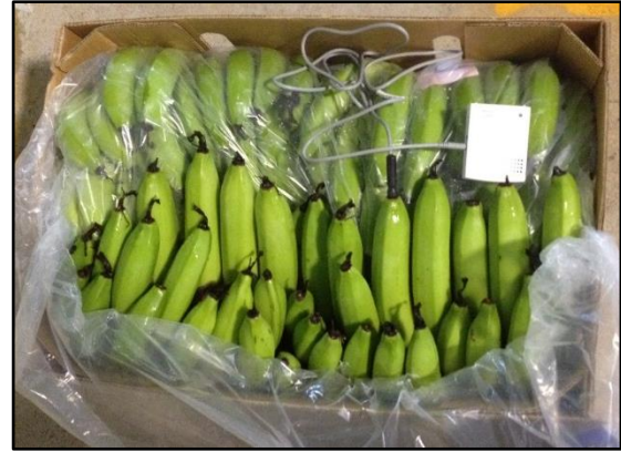
Figure 2. Data loggers placed on top of fruit in selected cartons. Temperature probe inserted into pulp through the tip of fruit.
