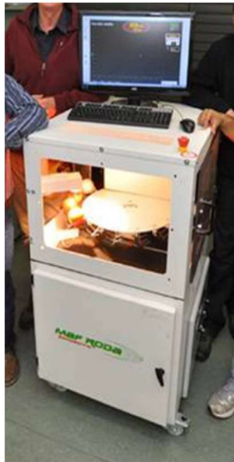
Figure 2. IDD2 test unit, from MAF Roda. Rotating carousel conveys fruit into light protected box for light transmission measurements.
