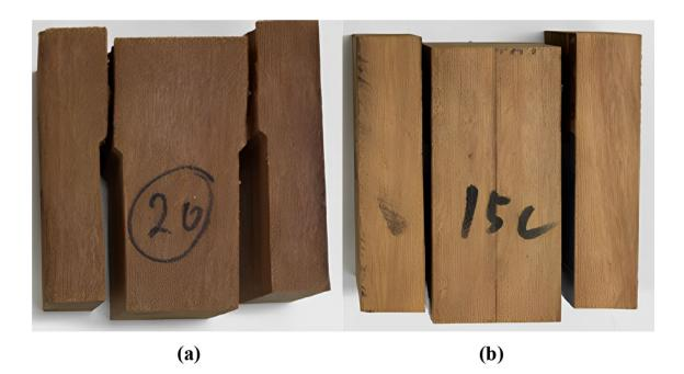
Fig. 14 Fracture Mode II typical failure modes for a TL and b glueline crack systems
