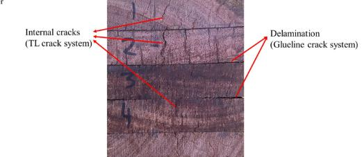
2017), designing the glulam with boards stacked in a specific grain orientation combination could improve the outcomes of the delamination test. Second, cutting stress relief grooves with specific shapes and arrangements in the boards could reduce the internal stresses (Raftery and Whelan 2014). Third, adjusting the board geometry (the width to thickness ratio) could affect the internal stresses and thus decrease the stresses imposed on the gluelines during the delamination test.
