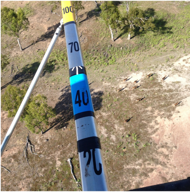
Fig. 3. Chital deer group (or cluster) passing under a survey boom attached to a Robinson R44 helicopter. Numbers on the boom refer to distance intervals on the ground perpendicular to the helicopter. Photograph credit: M. Amos.
