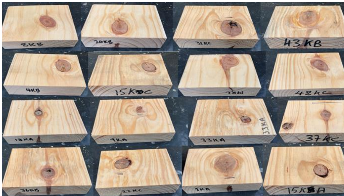
Figure 3. Examples of sound centred knots in samples.
