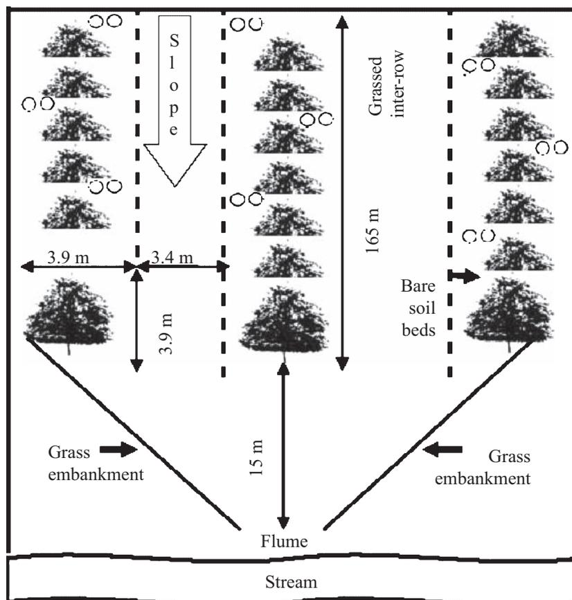
**Fig. 1.** Depiction of the 0.24-ha macadamia catchment used in the study (not to scale), showing the planting configuration of trees within bare soil beds, the adjacent grassed inter-rows, and the runoff collection flume positioned at the edge of the farm and alongside the catchment stream. Soil sampling points within the raised beds are depicted by circles (O O). Sampling points in the grassed inter-row are not-displayed.
