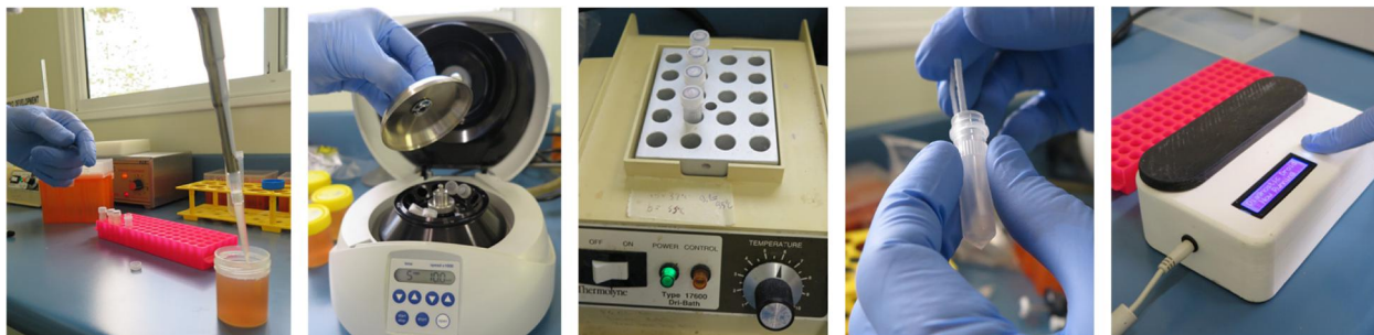
Fig. 1. Work flow for the Campylobacter Point-of-Management assay. A 2 mL aliquot of the carcass rinse is centrifuged (5 min) and the pellet resuspended, treated with proteinase K and heated to lyse cells and release DNA. The two cellulose dipsticks are added to the crude lysate to bind the released DNA. The dipsticks are then placed in a wash buffer and then in the LAMP reaction mix (one for C. jejuni and one for C. coli ). The LAMP reactions proceed for 100 min at 65°C in the 'Diagnostic Droid'. The Droid monitors the reaction and interprets the result.
