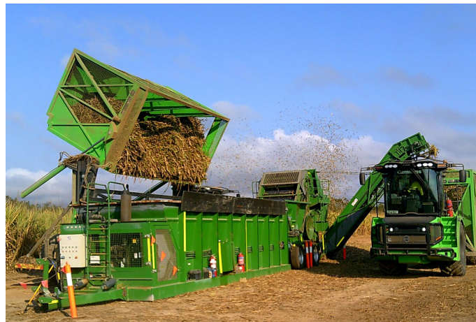
Figure 1. Norris ECT180 mobile cane cleaner and haulouts.
