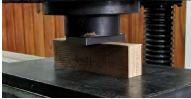
Fig. 5. Testing configuration for bearing strength perpendicular to the grain
