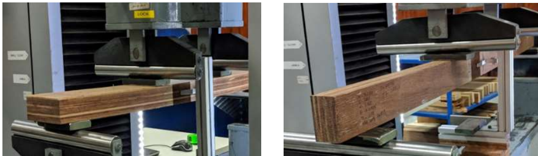
Fig. 4. Testing configuration for flatwise (left) and edgewise bending (right)
