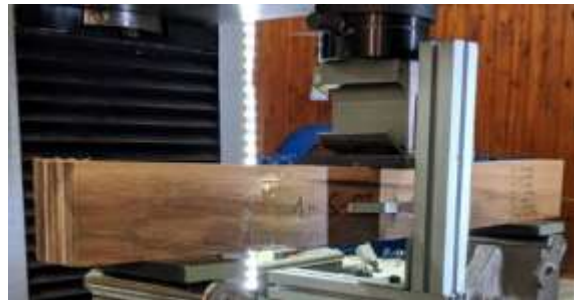
Fig. 7. Testing configuration for longitudinal shear strength
