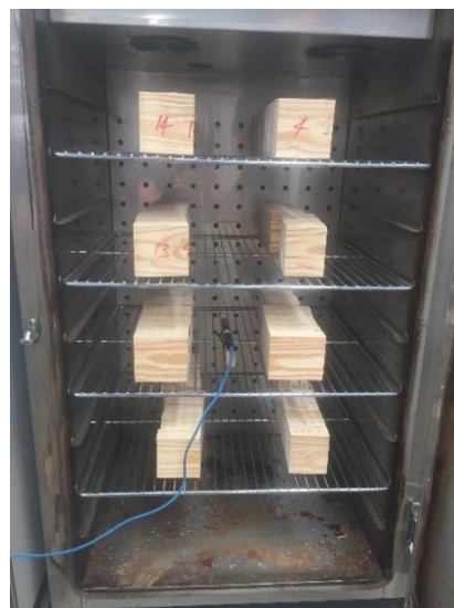
Fig. 2. Airflow measured in dehydrating oven with flow controlled through exhaust vent
