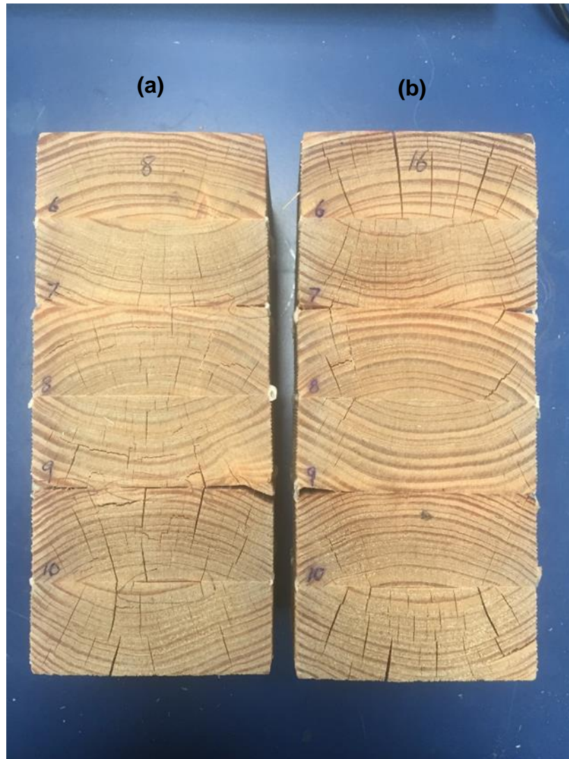
Fig. 10. (a) Specimens dried in the drying chamber exhibited a more uniform checking pattern than (b) those dried in the dehydrating oven. A central zone was easily identified where no checking had occurred.
