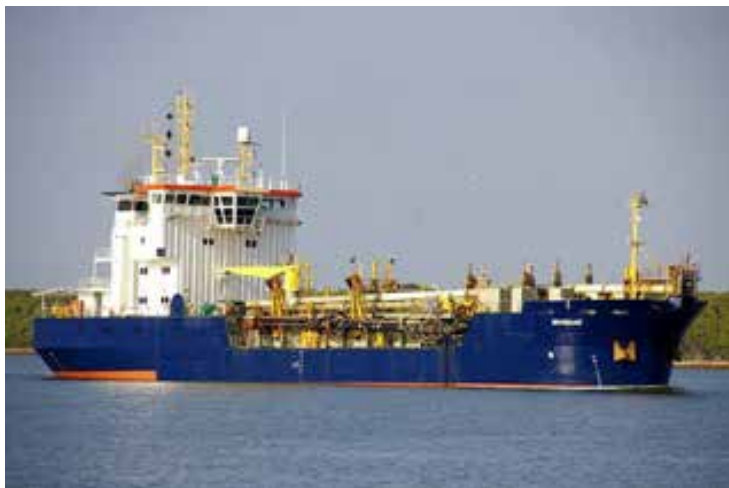
Figure 4. Port of Brisbane Pty Ltd trailer suction hopper dredge, Brisbane (image from Dredgepoint.org).
