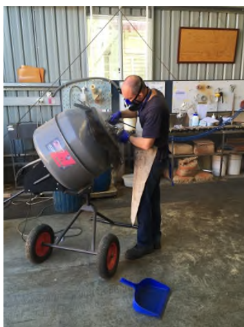
Image 5 – Using a rotary mixer for resinating and minimising fibre loss
