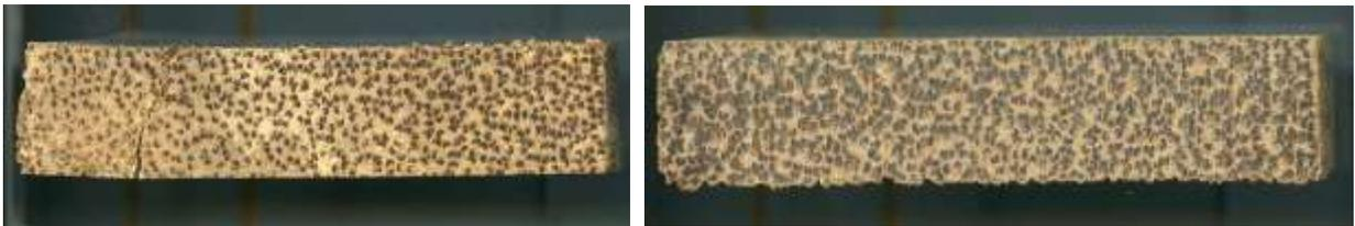
**Fig. 6.** End grain view of high density cocowood test specimens with densities of 866.5 kg/m<sup>3</sup> (L) and 1003.5 kg/m<sup>3</sup> (R) after exposure to *C. acinaciformis* and *M. darwiniensis*, respectively
