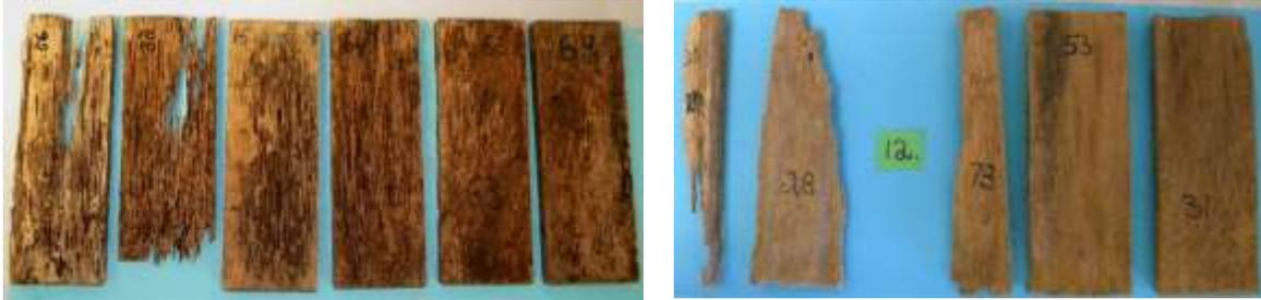
**Fig. 5.** Cocowood test specimens of increasing density after exposure to *C. acinaciformis* (298-938 kg/m<sup>3</sup>) (L) and *M. darwiniensis* (380-963 kg/m<sup>3</sup>) (R) – test specimen 12 was destroyed
