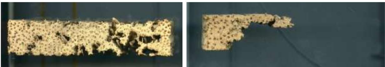
**Fig. 7.** End grain view of cocowood test specimens with densities of 483 kg/m<sup>3</sup> (L) and 454 kg/m<sup>3</sup> (R) after exposure to *C. acinaciformis*
