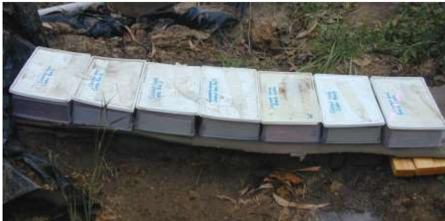
**Fig. 1.** Containers placed on top of bricks connected to a mound of *C. acinaciformis* near Townsville
