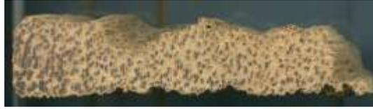
**Fig. 8.** End grain view of a cocowood test specimen (density 673 kg/m<sup>3</sup>) partially eaten by *M. darwiniensis* with a high concentration of vascular bundles in the uneaten portion
