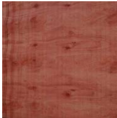
A veneer sheet peeled from 13 year-old plantation-grown wood.
