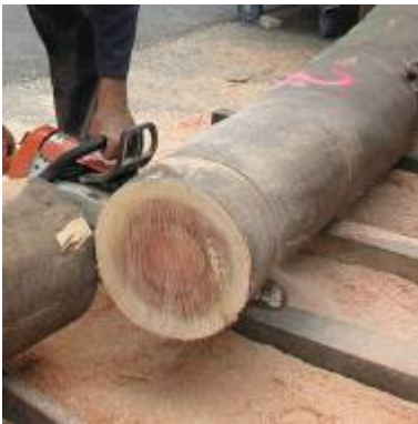
A 13 year-old, de-barked red mahogany log showing the typical proportion and colour of the heartwood.
