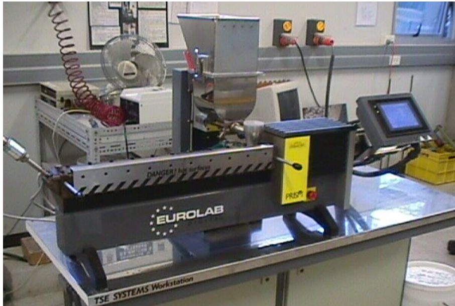
Figure 1. Prism Eurolab KX16 twin screw extruder used for prawn meal diet extrusion trials.
