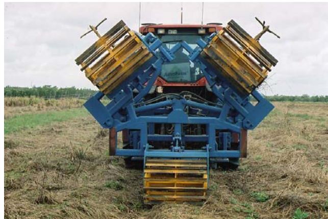
Figure 5: Russo Bros. Zonal Tiller; folded for road transport
