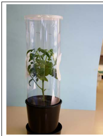
Photo 1. Cylindrical film cage set-up used to assess adult mortality
