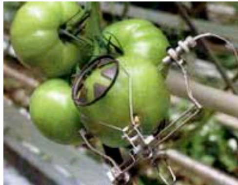
Figure 2 left: Photograph of the Phytech stem diameter sensor monitoring a capsicum plant and Figure 3 below: a fruit (or bulb) diameter sensor in greenhouse tomatoes. (Photographs supplied by VP Marketing, PhyTech Ltd.)
