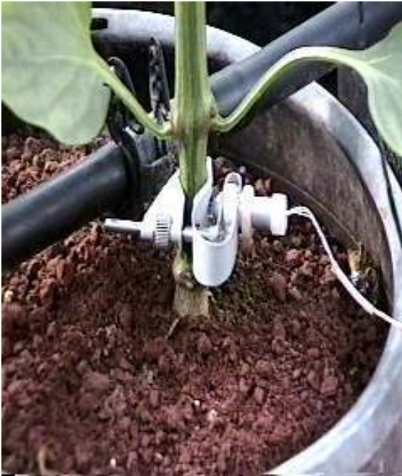
Figure 2 left: Photograph of the Phytech stem diameter sensor monitoring a capsicum plant and Figure 3 below: a fruit (or bulb) diameter sensor in greenhouse tomatoes. (Photographs supplied by VP Marketing, PhyTech Ltd.)
