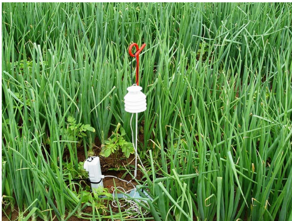
Figure 1: The Phytech monitoring system in an onion crop (Photograph supplied by M. Cutting)
