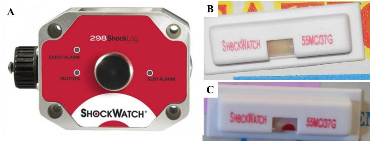
**Fig. 2.9** A: A ShockLog device used to record impact magnitudes and events (<http://www.shockwatch.com/products/impact-recorders/shocklog-298/>). B: An un-triggered impact indicator clip of 37G attached to an avocado fruit tray. C: An impact indicator clip that has changed colour to red due to an imposed impact event above the threshold limit.
