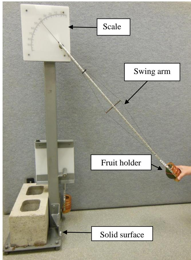
**Fig. 2.2** Individual avocado fruit drop equipment. A single fruit was placed in the holder attached at the distal end of the swinging arm. The fruit was raised to the desired drop height for release and free fall onto the solid metal plate surface. The rebound height of fruit was observed against the measuring scale and recorded.
