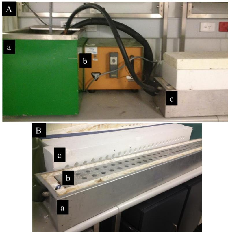
**Fig. 2.6** A: Temperature gradient block set up with associated apparatus; a) chilled water bath unit, b) refrigeration unit, and c) the temperature gradient block. B: a) Temperature gradient block with; b) drilled holes in positions ranging from low temperature (left) to higher temperature (right), and c) insulation. The far end is connected to a heating unit to maintain the higher temperature at desired level.
