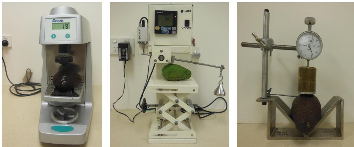
Fig. 1: Avocado cv. Hass fruit firmness measurement with the Sinclair Internal Quality Firmness tester (left), the Electronic Firmometer (centre) and the Analogue Firmness Meter (right).
