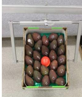
Impact recording device and shock loggers were used in these experiments for their calibration for further use in the supply chain studies.
