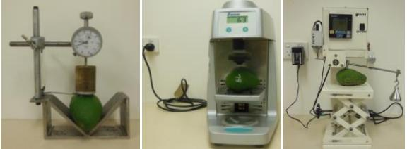
Measurement of fruit firmness with analogue firmness meter (Left), SIQ firmness tester (Middle), and electronic firmometer (Right)
