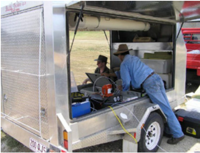
Figure 10. Initial on-site biogas analysis using a Teledyne Chemiluminescence H 2 S analyser installed in trailer.
