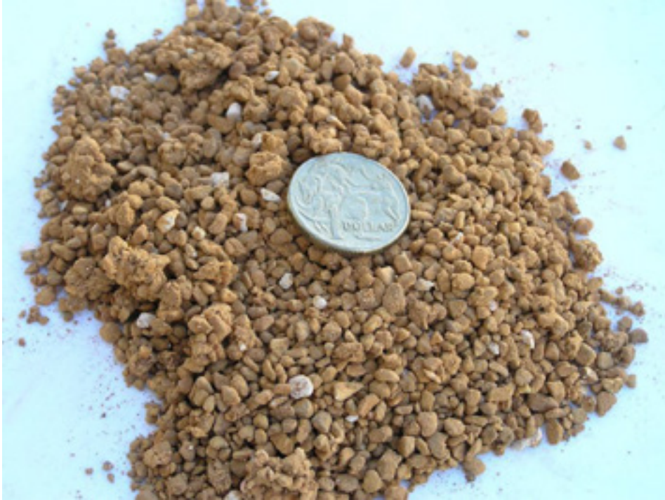
Figure 7. A photograph of the SULFA-BIND® proprietary H 2 S adsorption medium to be trialled in the down-flow biogas scrubber.
