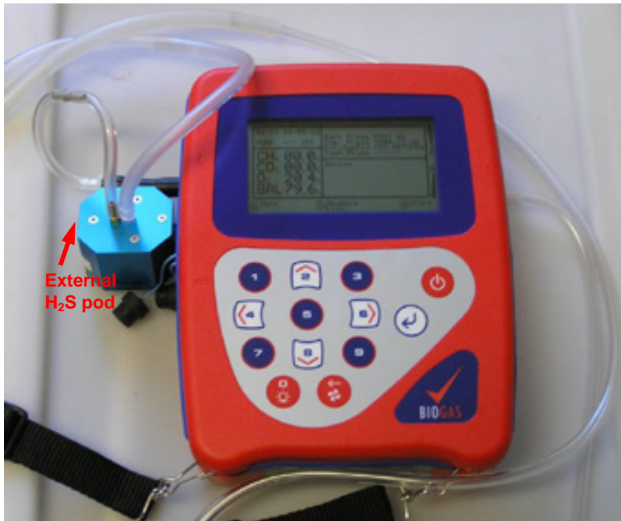
Figure 12. Geotech Biogas Check portable gas analyser used to monitor biogas quality and scrubber performance.
