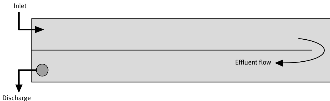
Figure 2. A plug-flow lagoon design, which prevents short-circuiting of flow between inlet and outlet, is most appropriate for DWT.
