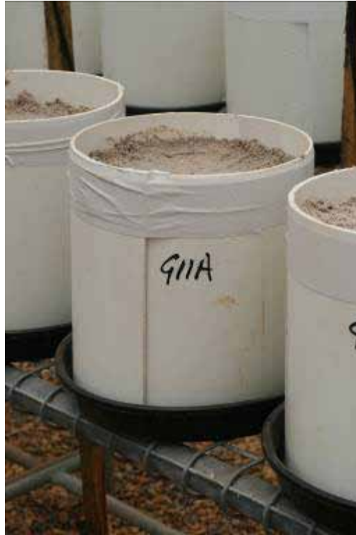
Plate 2 - Split columns enabled access to roots for examination and assessment of root mass.
