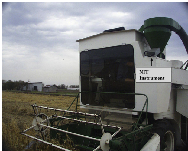
Fig. 1. NIT instrument mounted on the side of the grain collection hopper.
