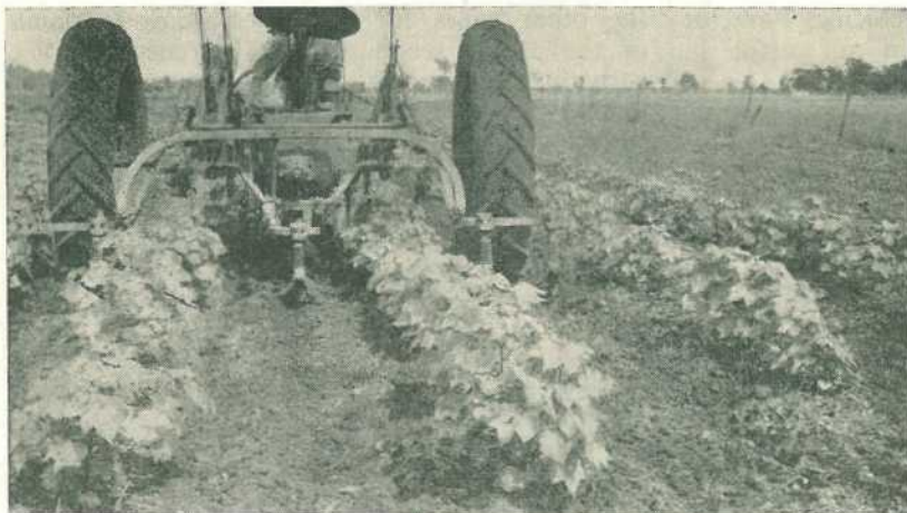
Plate 5 High-Clearance Scarifier Suitable for Late Cultivation.
