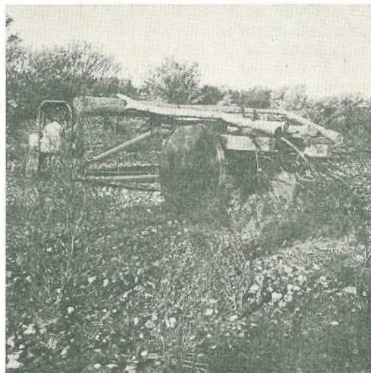
A 'mulga basher' in use in the Quilpie district. These machines are useful in open stands of mulga and allow the use of smaller tractors for feeding stock.
