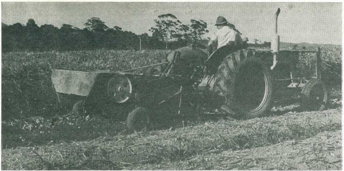
Late harvest of ginger using an adapted potato digger.
