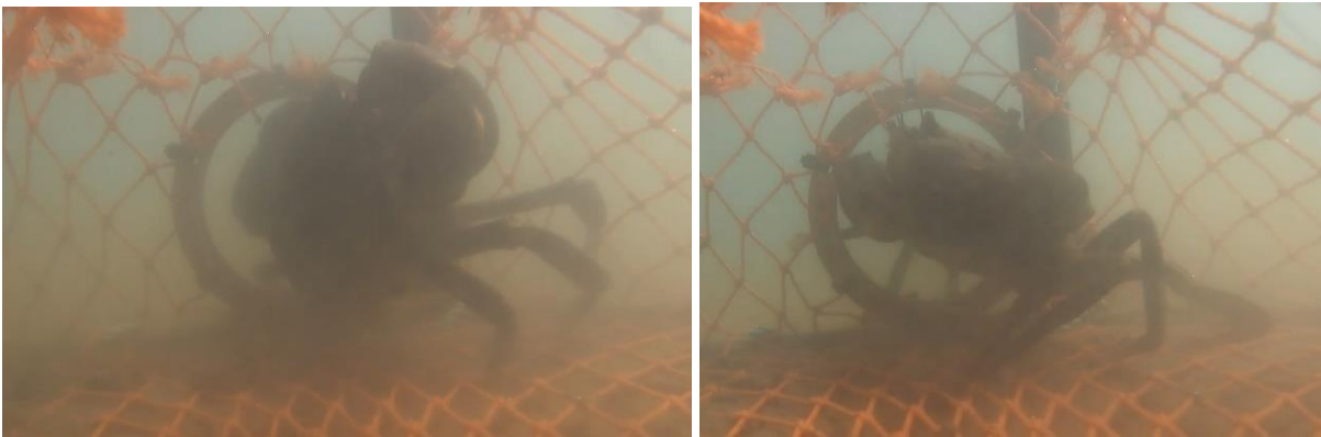
Figure 24. Underwater image of a male Giant Mud Crab exiting via a 105 mm round escape vent that has a 20 mm border.
