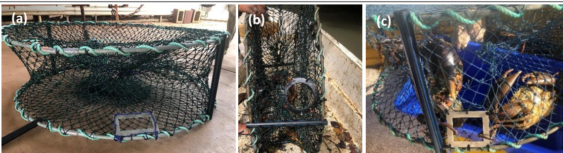
Figure 1. Escape vents in commercial crab pots: (a) large rectangular 120 x 50 mm; (b) round 105 mm diameter (internal); and (c) two small rectangular of a least 75 x 60 mm.
