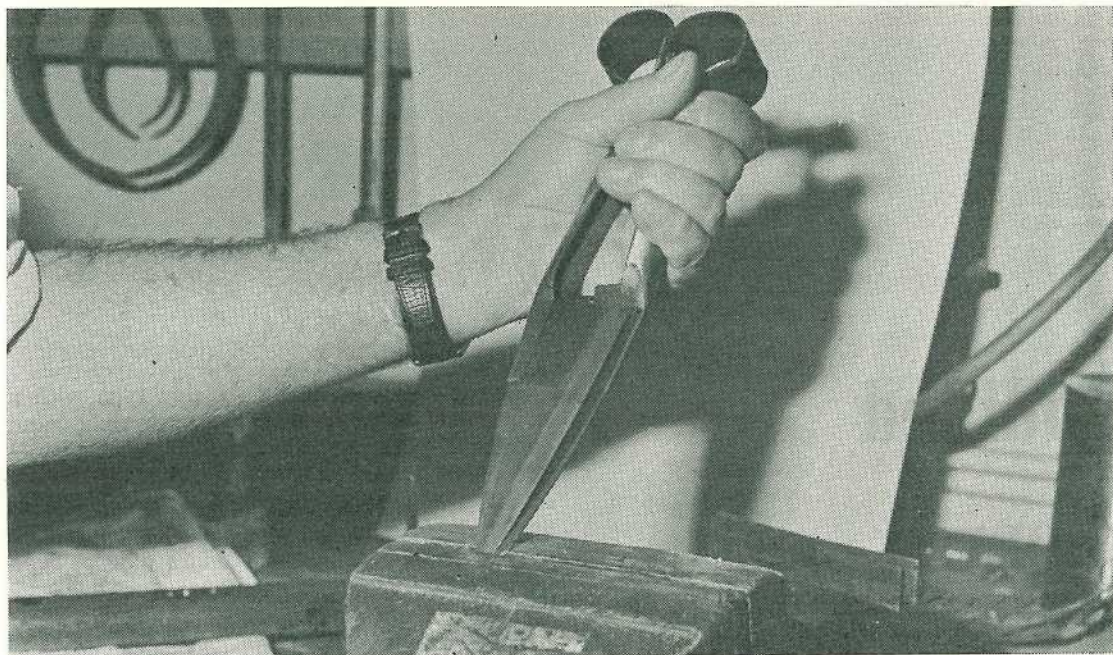
Breaking points off and reducing length of blade by 6 mm. Ends should be bevelled to a rounded blunt point.
