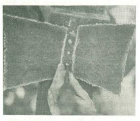
Plate 7. The holes for the keeper and tongue should be marked with a centre punch and drilled before any bends are made.
