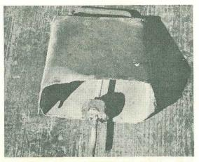
Plate 10. A heavy nut makes a good hammer. The hammer is in the correct position when its bottom edge is 2 to 3 mm below the bottom edge of the bell.
