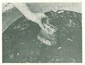
Plate 11. Dip the bell open end first into water to check that there are no holes in it. Holes must be filled with braze.
