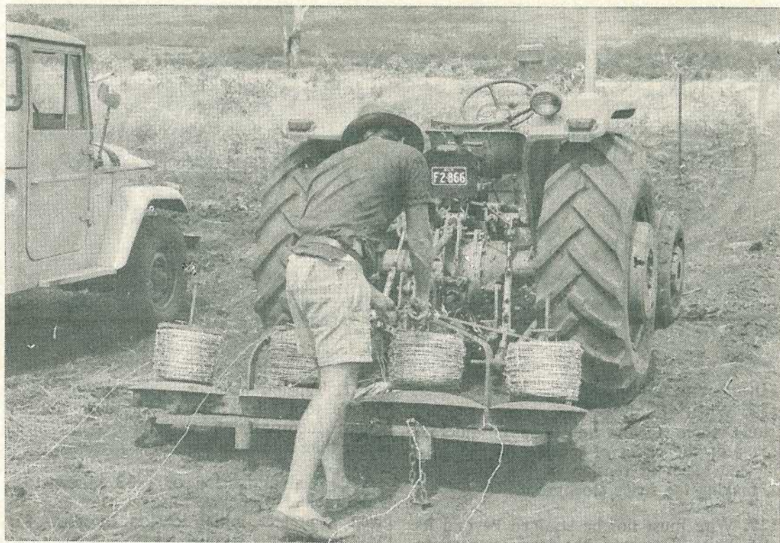
A simplified barb wire running machine mounted on the carry-all of a tractor.
