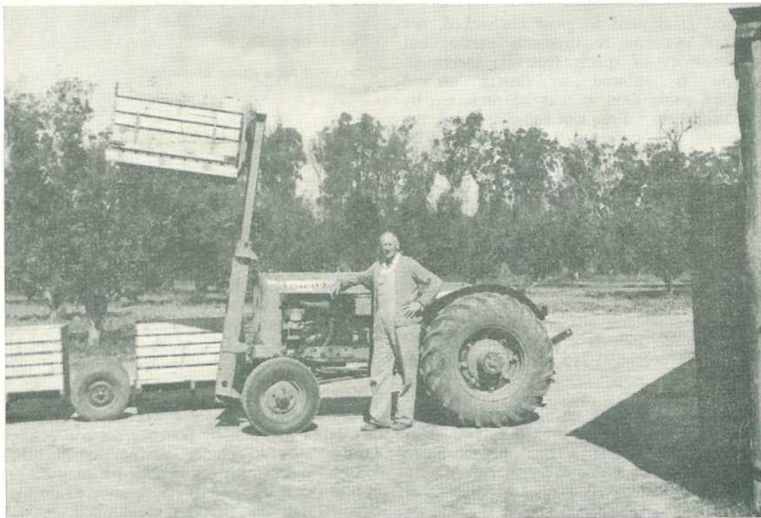
BELOW. Fork-lift attachment on a tractor used for handling bulk bins.
