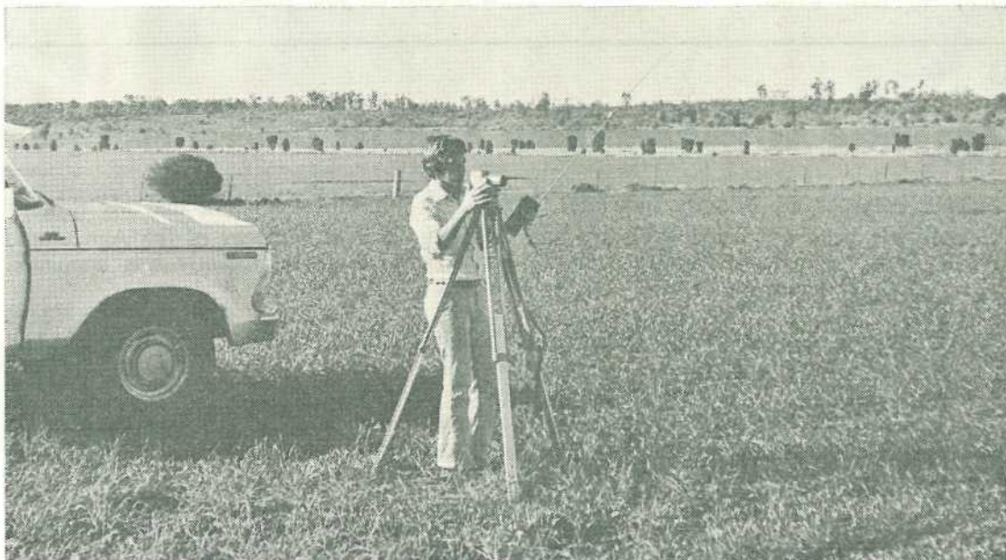
Above and Below. Surveying and marking contour lines for grass strips or as preparation for a parallel system using a mobile staff.
