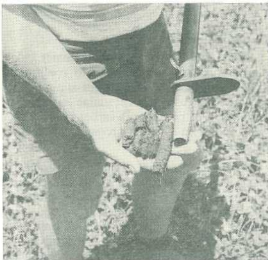
Soil cores obtained using a tapered tube soil sampler.
