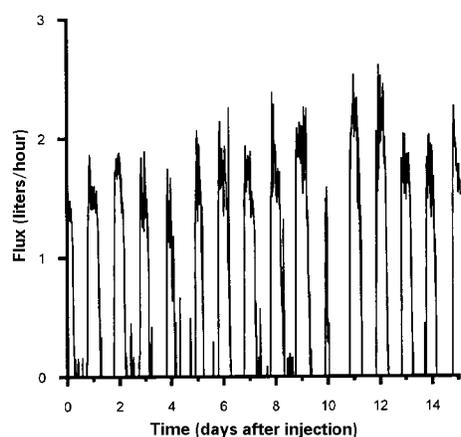
Figure 2. Sap flux estimated by the heat pulse method for Tree T6 at Toolara ( $t = 0$  represents noon on the day of injection).
