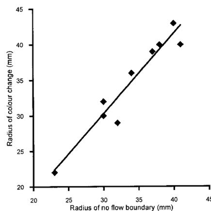
Figure 1. Radius of no-flow boundary determined by the heat pulse method versus mean radius of sapwood conducting area for each tree at Toolara. The  $r^2 = 0.93$  ( $y = 1.13 (\pm 0.08)x - 3.62 (\pm 2.96)$ ).
