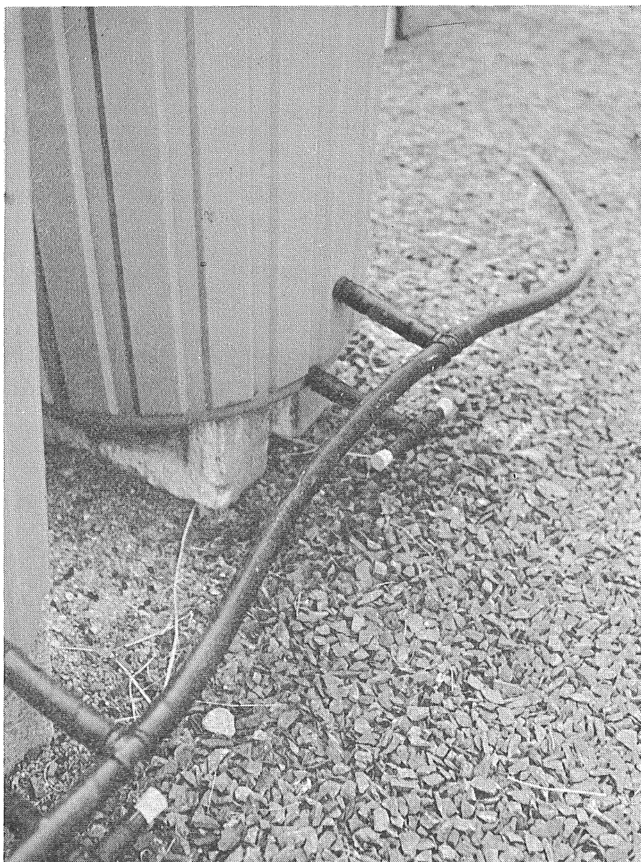
Fig. 4.—Lower parts of pots, showing upper outlets leading to bottom reservoir and stoppered lower outlets.
