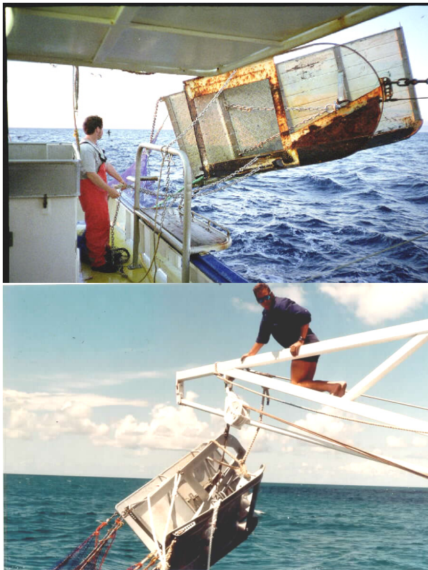
Figure 5.4.13 Types of otter boards used in the Queensland east coast trawl fishery. Above is large flat otter board with skid, as used in triple gear in deep water eastern king prawn fishery. Below are two Bison boards with skid in between, used in quad gear in the tiger/endeavour prawn fishery.
