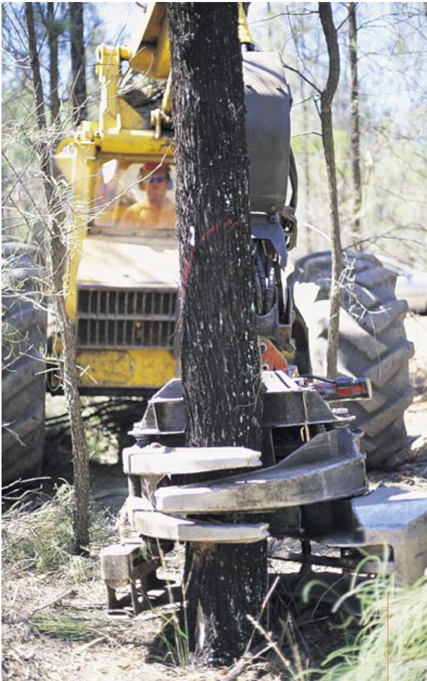
Contractor Ken Murray harvests cypress pine in the Dalby forestry district with a Bell harvester. This harvester reduces environmental impacts on the surrounding forest by giving the operator greater control over falling trees.
