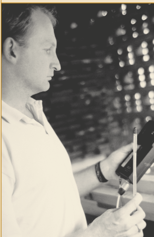
Senior Timber Technician Gary Hopewell using a wind speed analyser in a solar kiln.
