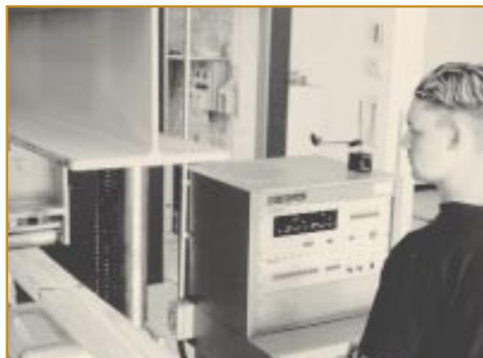
Technical Assistant Matthew Craven uses the Queensland Forestry Research Institute-developed universal timber strength tester. Through QFRI, DPI Forestry continues to improve timber processing technology.
