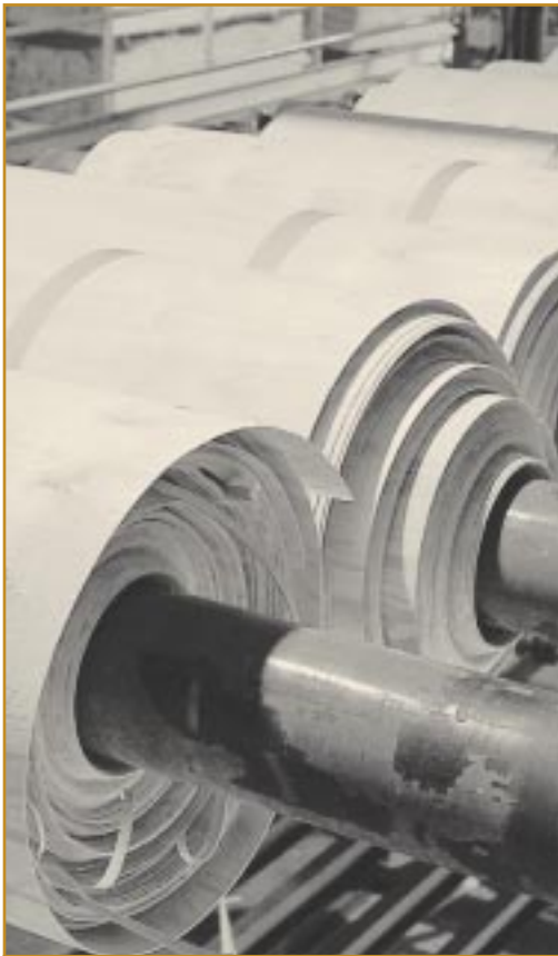
Rolls of Araucaria cunninghamii peeled from hoop pine logs at D.G. Brims & Sons sawmill at Yeerongpilly are turned into hoop pine plywood boards.
