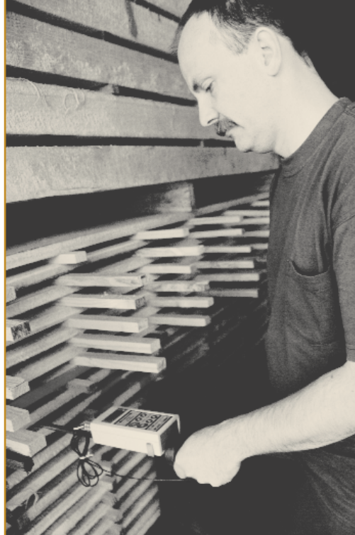
Research Scientist Waldemar "Waldec" Bartnikowski, with a QFRI developed moisture metre. Through QFRI, DPI Forestry continued a range of cooperative research and development programs with Queensland's timber industry.
