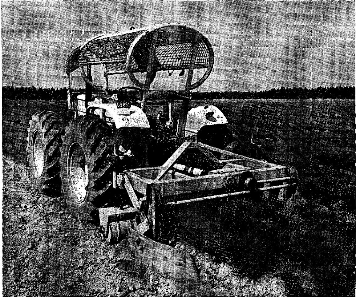
Root pruning Slash Pine in Toolara nursery using a departmentally designed and constructed reciprocating unit.
