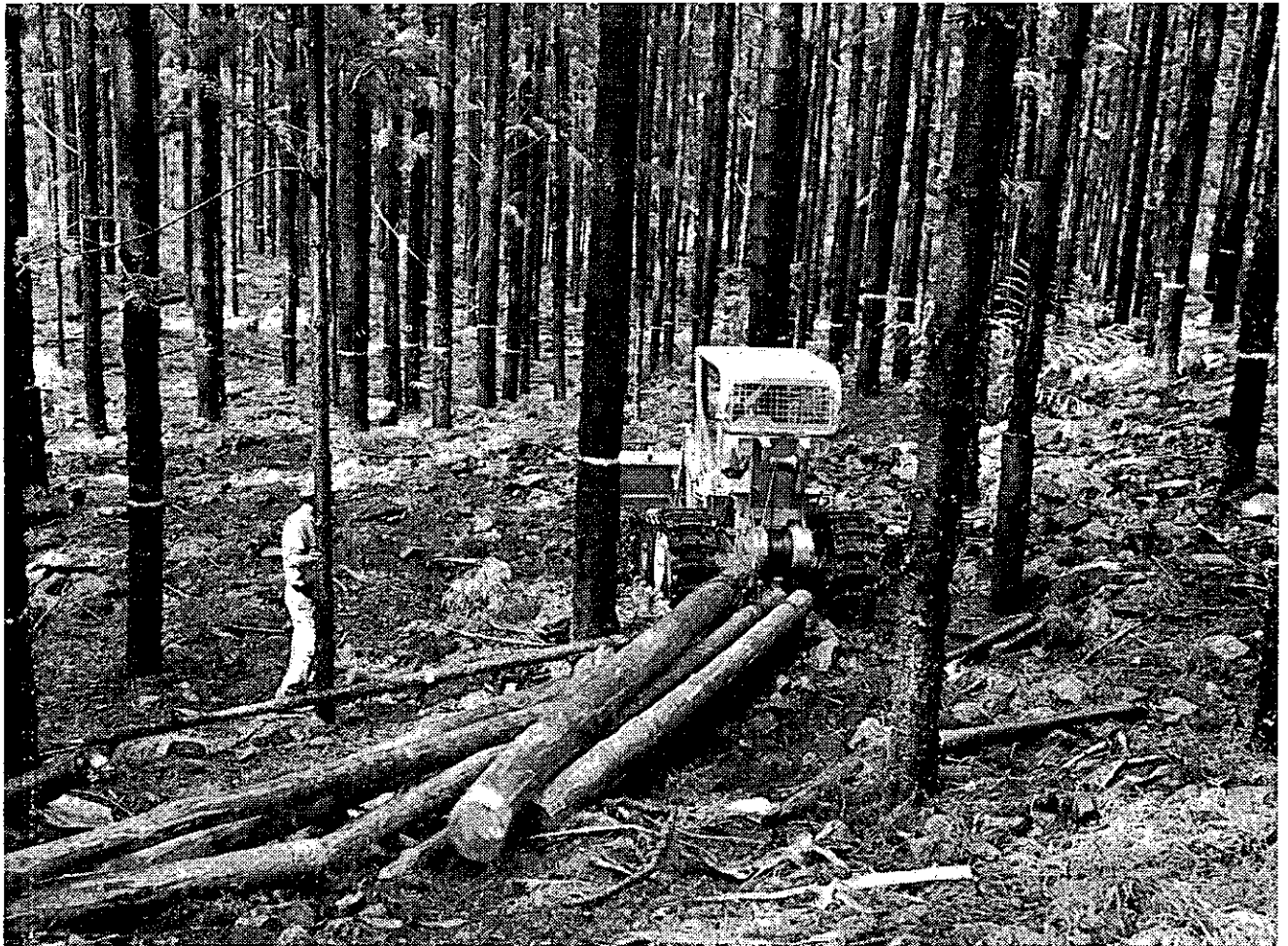
TRACTOR SNIGGING IN HOOP PINE PLANTATION, AMAMOOR. Tractor snigging is becoming general practice with Plantation Thinnings. A record 49 million super. feet of these thinnings were logged during the year.
