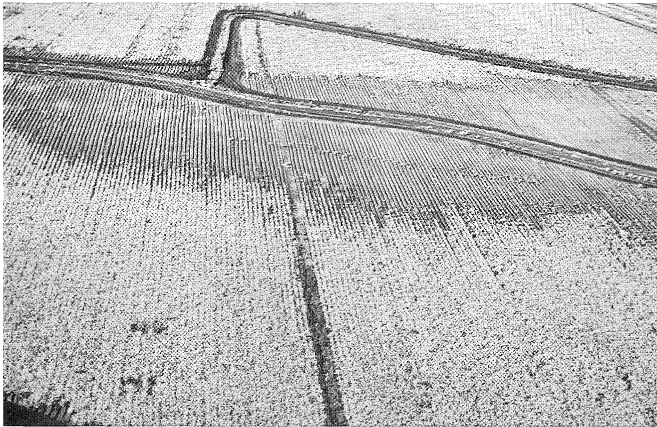
Some 200 ha of the Emerald Irrigation Area have been affected by high salinity due to shallow water tables. In one of these areas (the dark patch on the picture), shallow drains are slowly reclaiming the soil for cotton growing.
