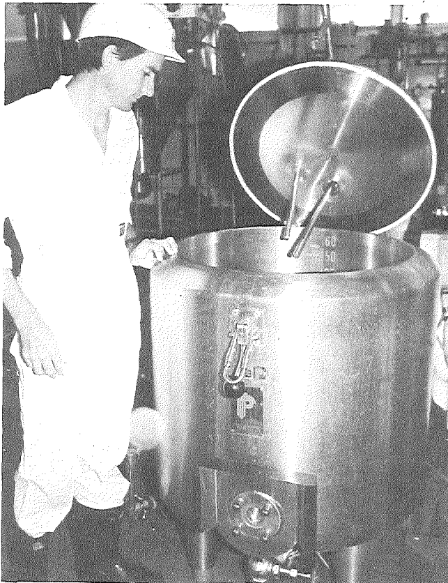
The fermentation vat for cultured milk at the Otto Madsen Dairy Research Laboratory.
