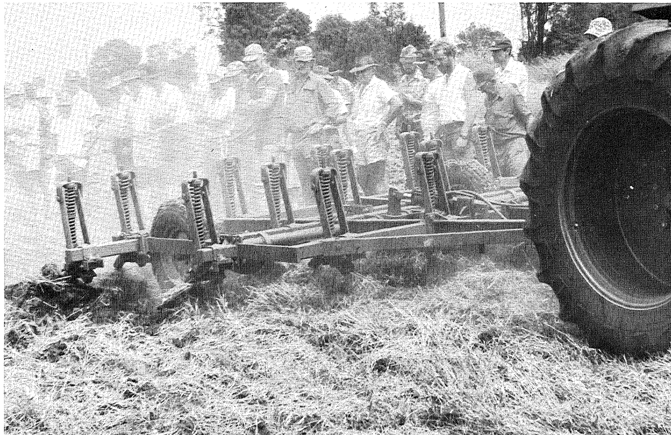
Farmers inspect the trash handling ability of a modern chisel plough demonstrated at a field day conducted by the DPI South Burnett Crop Industry Committee at Wooroolin on 10 March.
