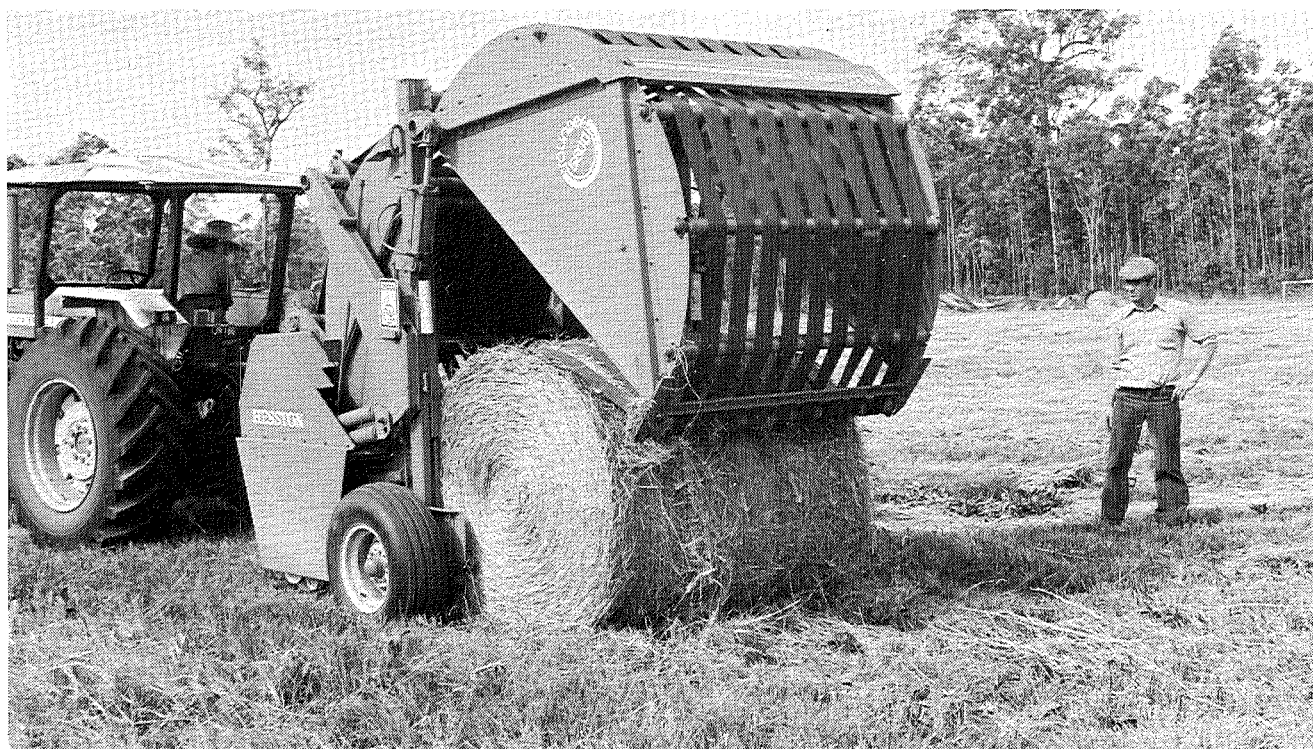
Large, round bales are suited to paddock storage of hay for on-farm use as they reduce weathering losses. This specialized machine is baling Rhodes grass after the seed had been harvested. It is working at Bauple, near Maryborough.
