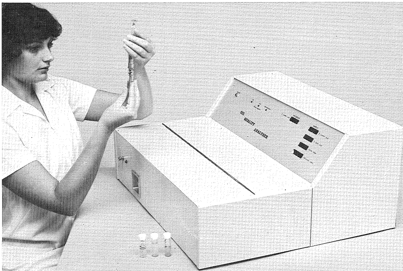
Lesley Ruddle, a technician with Agricultural Chemistry Branch, tests sunflower oil samples on the Oil Quality Analyser, an instrument designed and built at the Indooroopilly laboratories.
