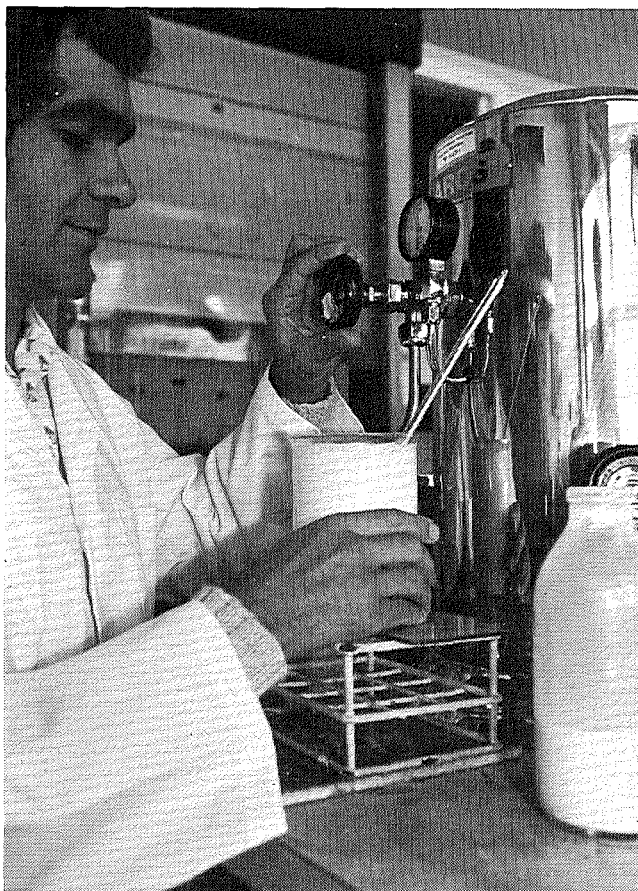
Sampling concentrate from the ultrafiltration pilot plant at the Otto Madsen Dairy Research Laboratory.
