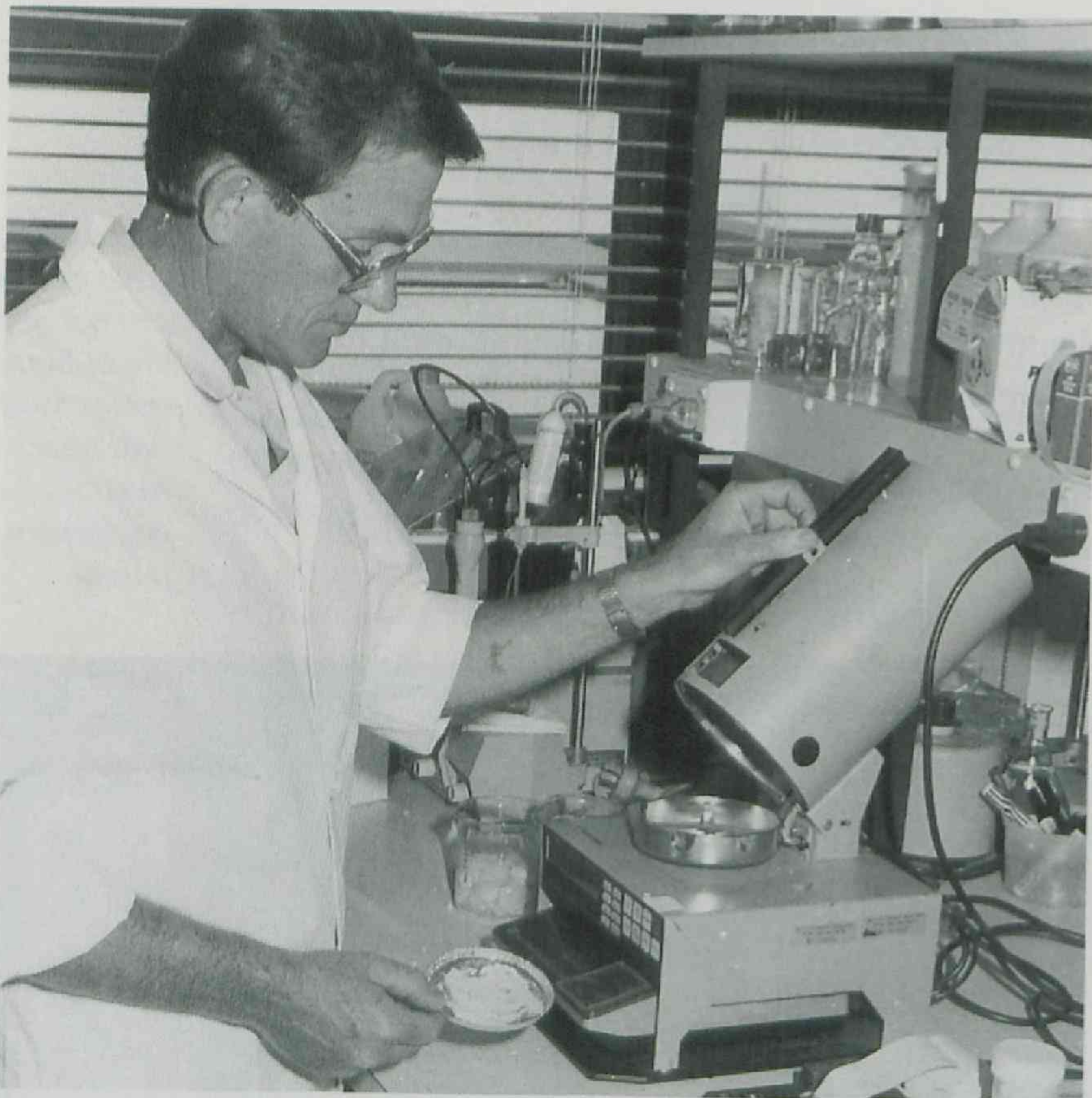
Seafood experimentalist Ross Smith uses an infrared moisture tester to measure the water content of scallops of different sizes and caught in different season to determine the natural variation. With this information it is possible to detect added water.
