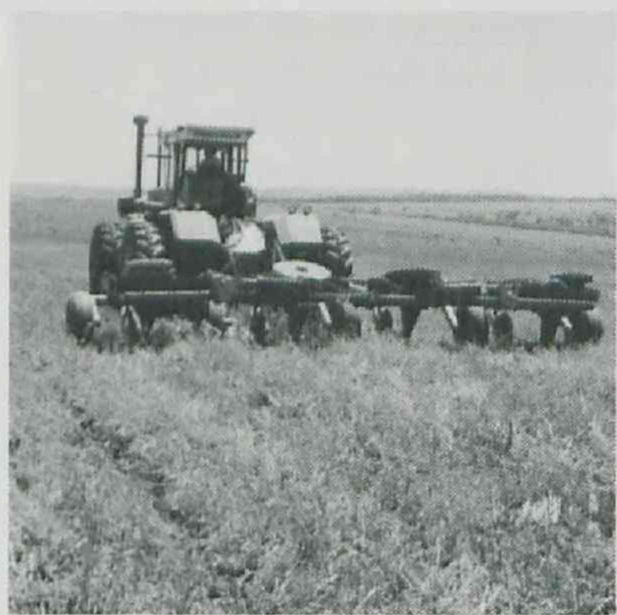
Stubble-mulching machinery, such as this blade plough, is used to cultivate the soil, with minimum disturbance. Plant residues are retained on the surface to protect the soil from erosion during heavy rain and to increase rainfall infiltration into the soil.
