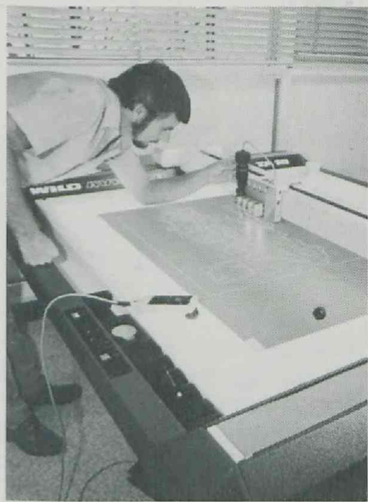
A cartographer uses a Wild TA10 flat-bed plotter for scribing thematic data in producing a soils map. The plotter is part of the recently installed computer-assisted drafting workstation installed in the DPI's land resources branch, Indooroopilly.
