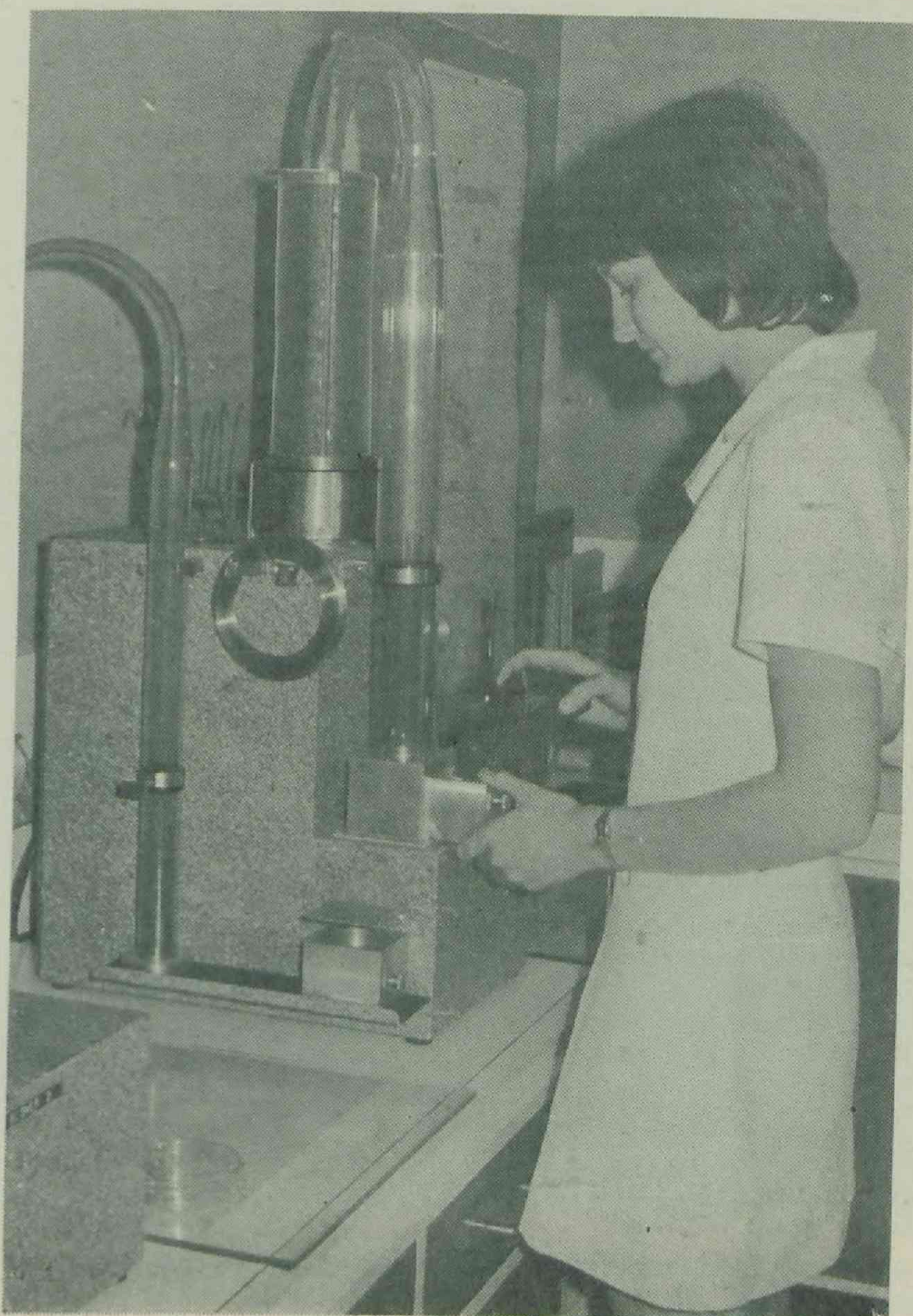
Operating a laboratory seed blower to remove lighter, inert material from a sample of pasture grass seed.
