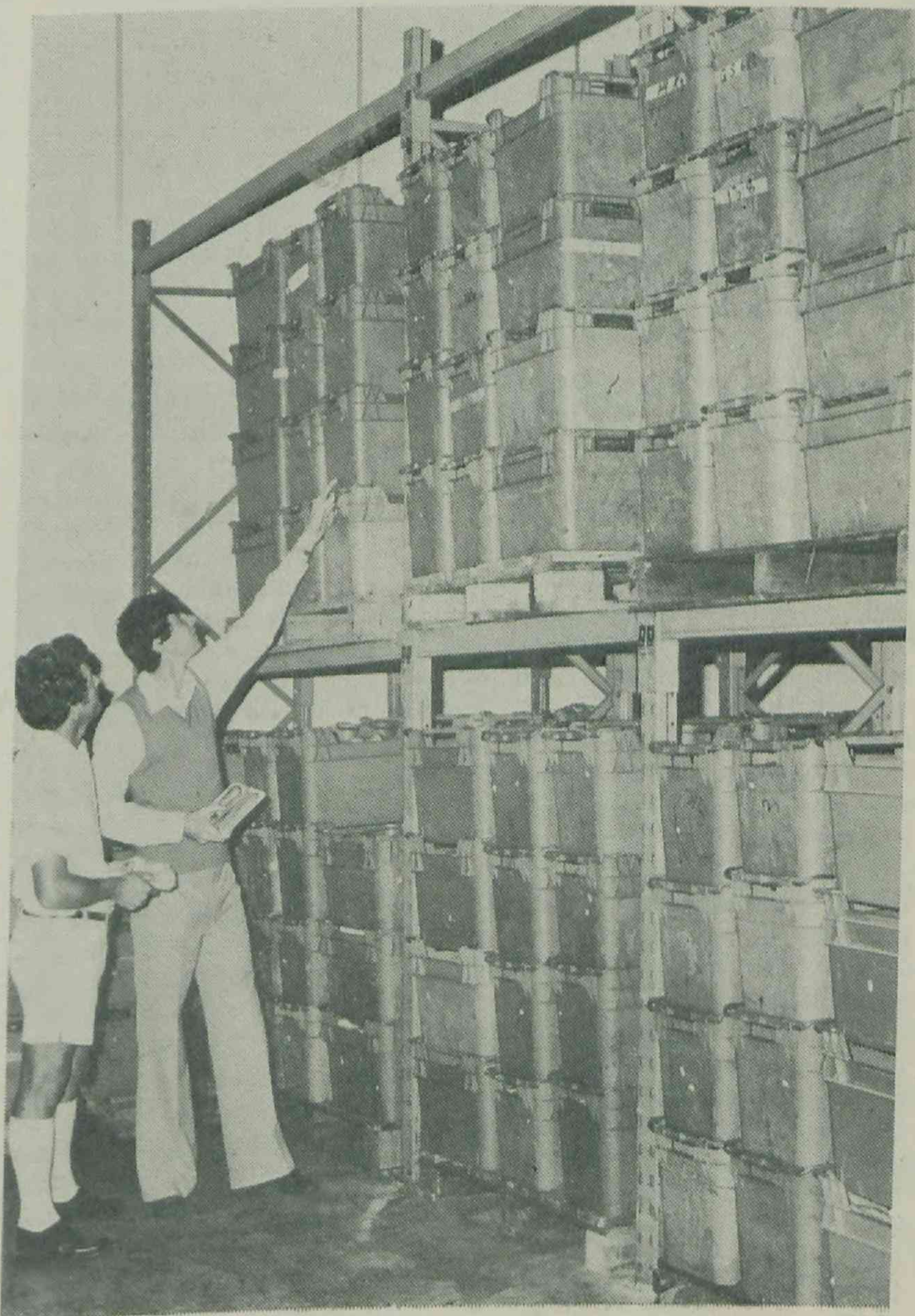
Pallet racking is the most efficient means yet devised for storing produce. Thirty-six-litre returnable crates are being used in this store.
