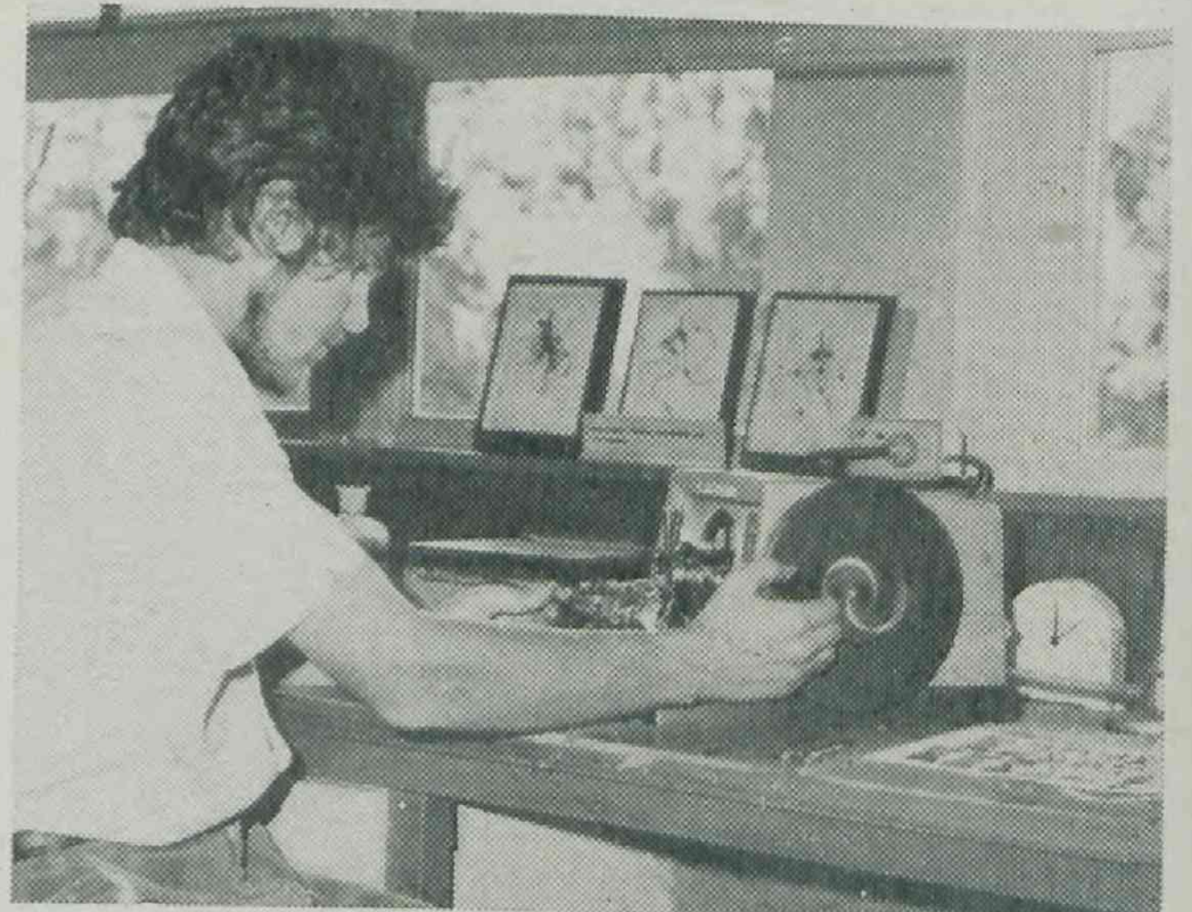
A microtome being used to cut thin sections of a nodule from the roots of a tropical legume for nematode studies.
