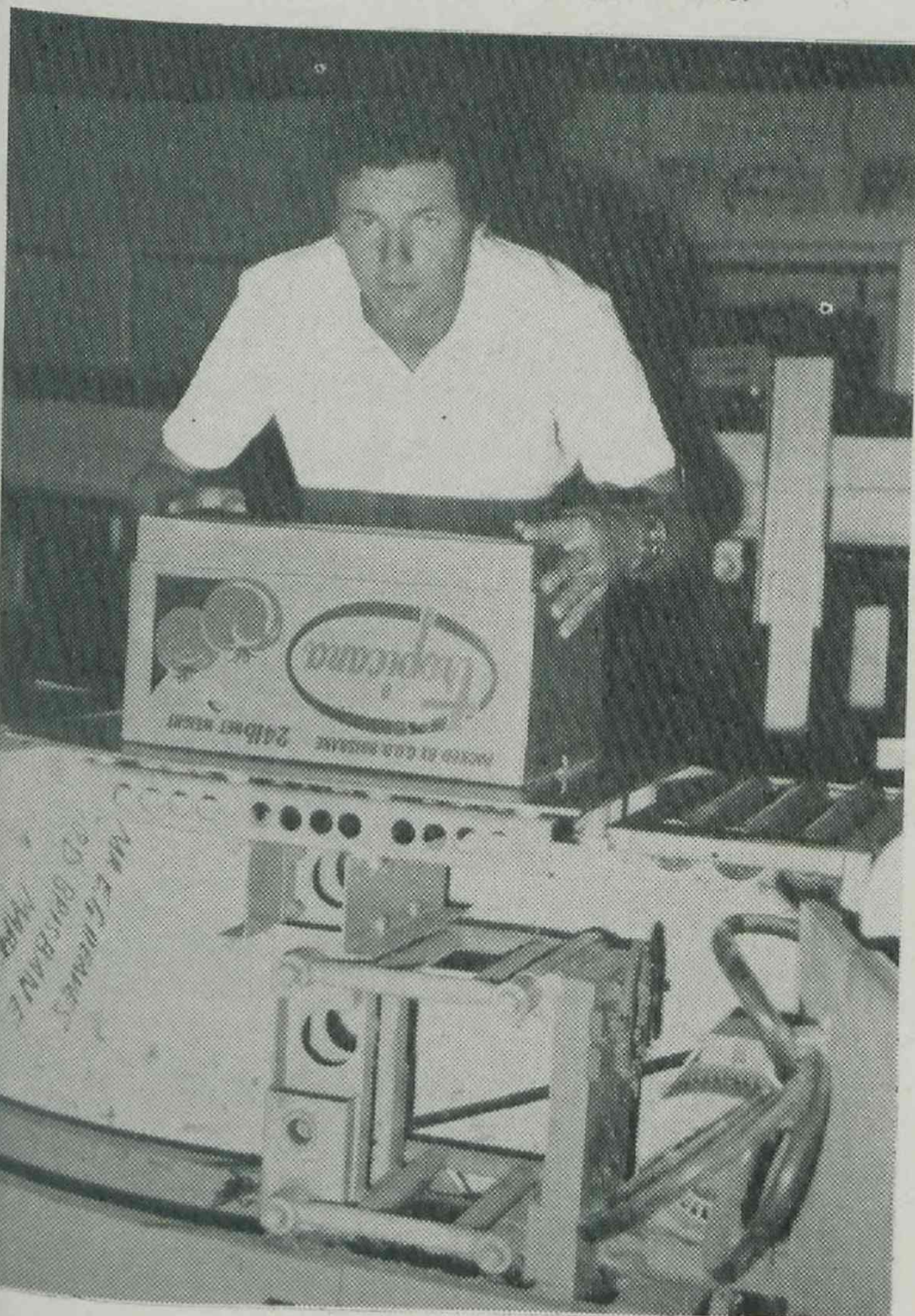
New packaging methods: a vibrator being used to produce a tight fill in a tomato packing line.
