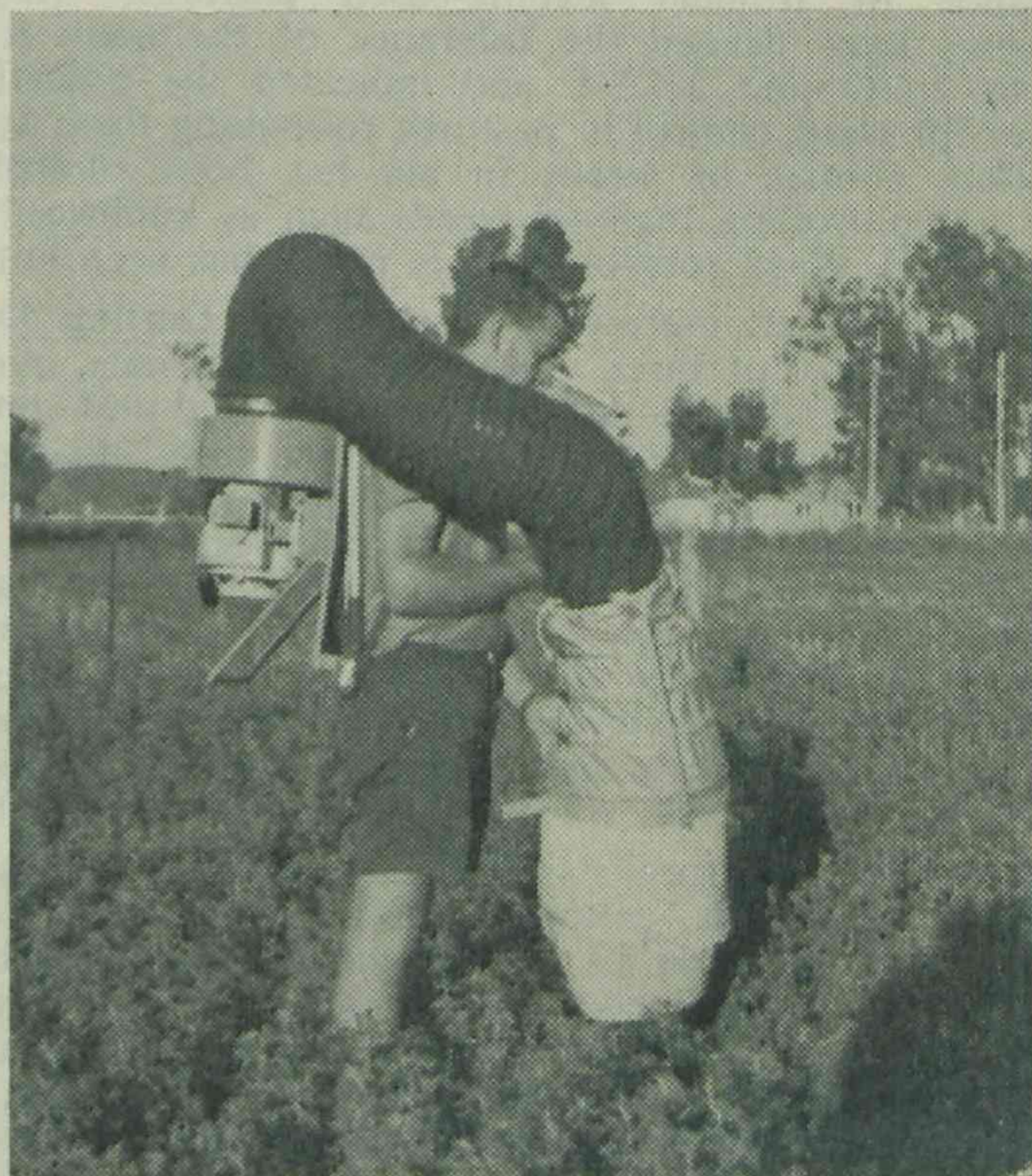
Large mechanical vacuum insect collecting machine for determining insect species and populations in field crops.
