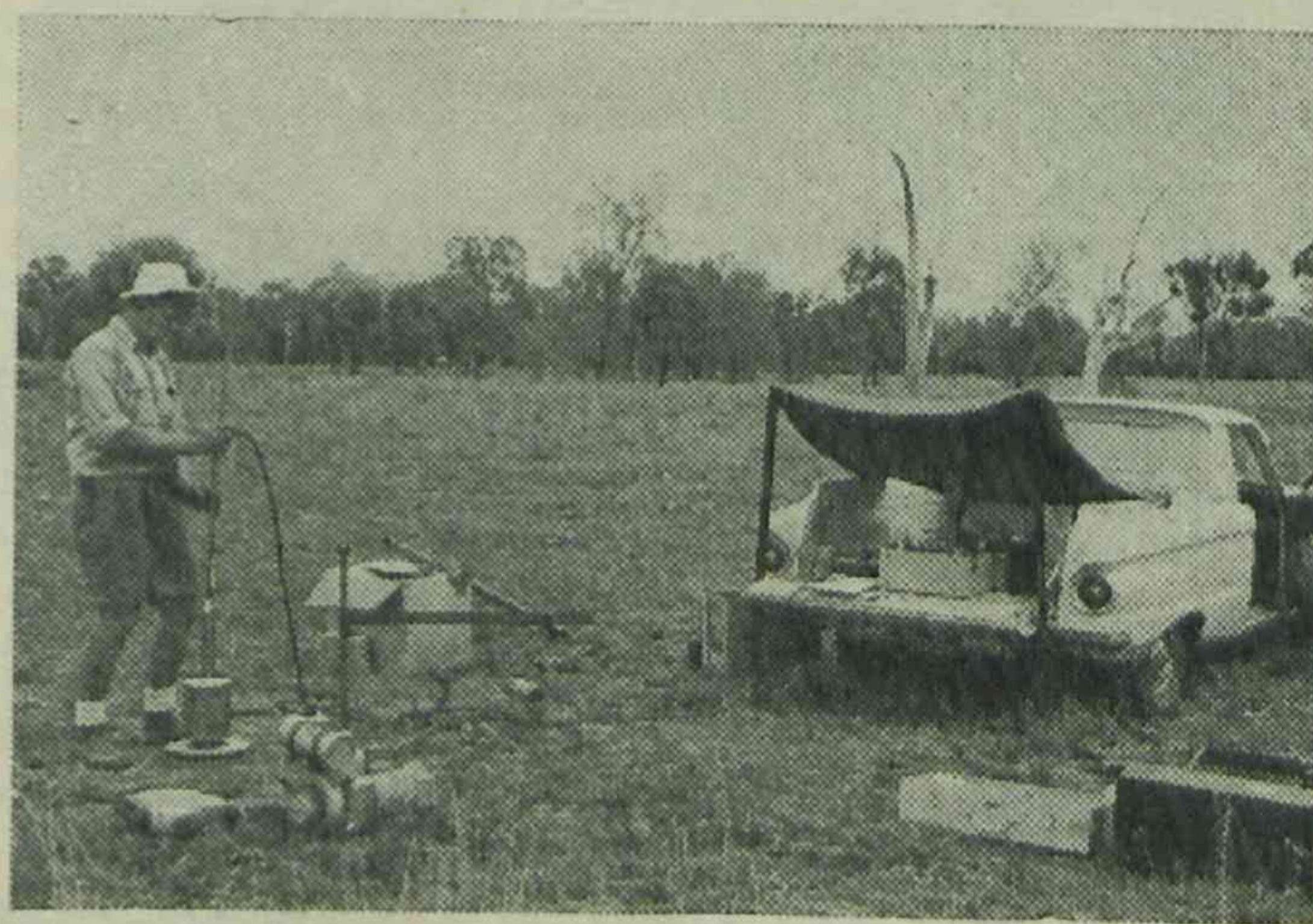
Field equipment such as this neutron soil moisture meter being calibrated by an agronomist is a great aid to irrigation and dryland studies.
