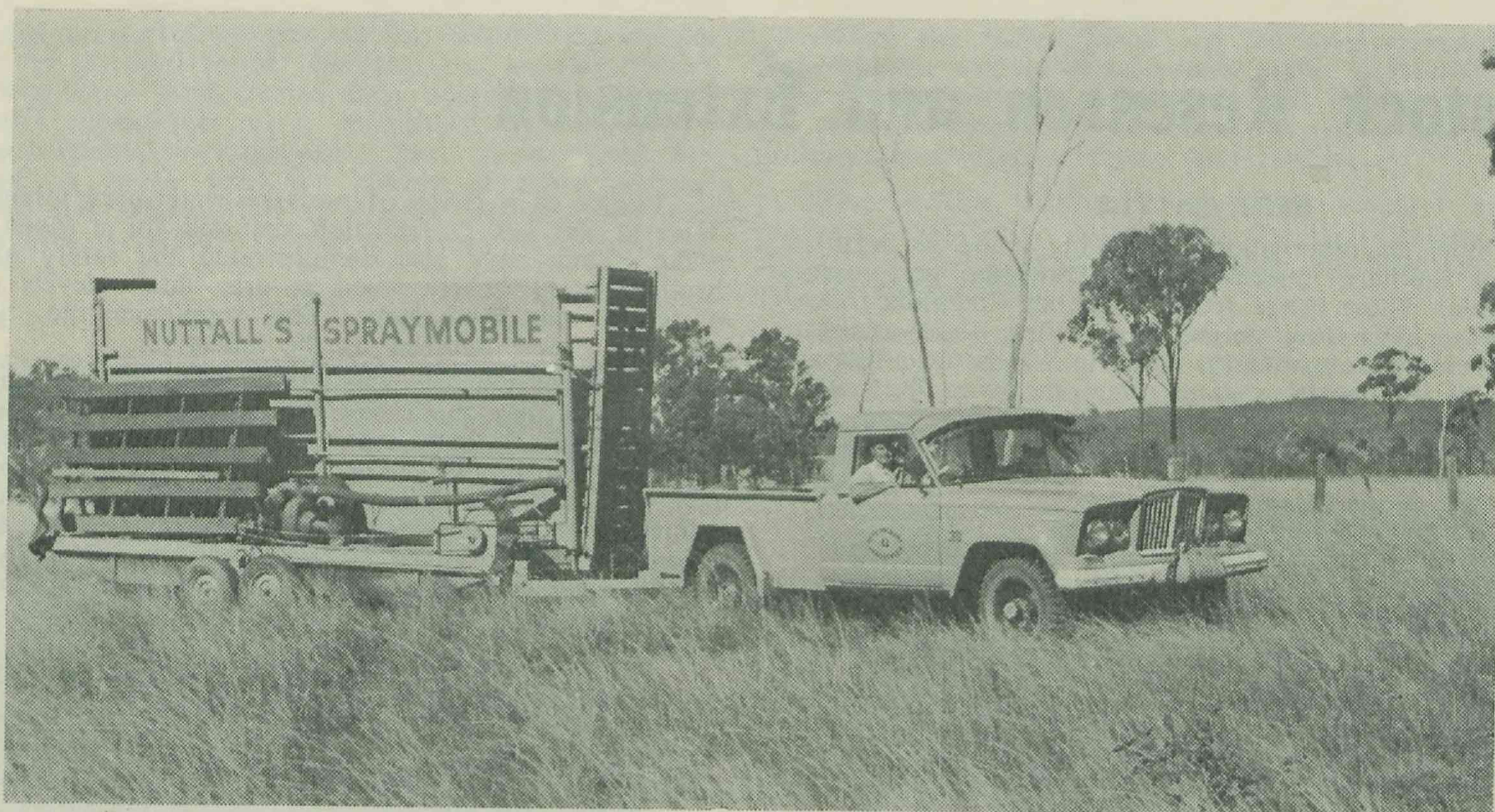
Mobile spraying unit designed by the Department for use in the resistant cattle tick control programme.
