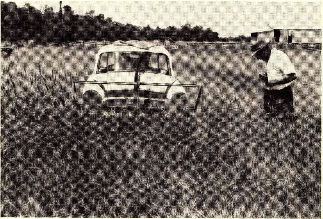
Plate 3.—A demonstration buffel grass seed harvester at work in a strain trial near Goondiwindi.
