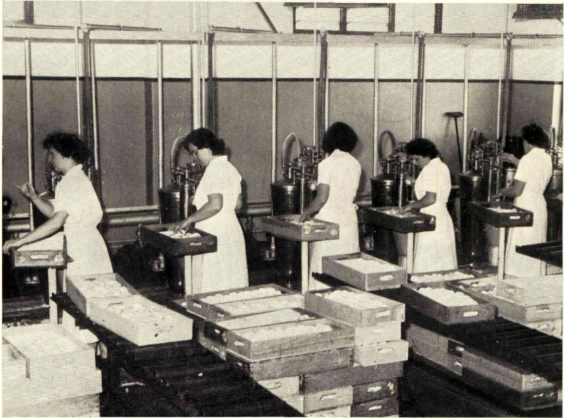
Plate 3.—A Section of the Battery of 20 Egg Pulp Vacuum Extractors in Operation at the Egg Marketing Board's Premises.
