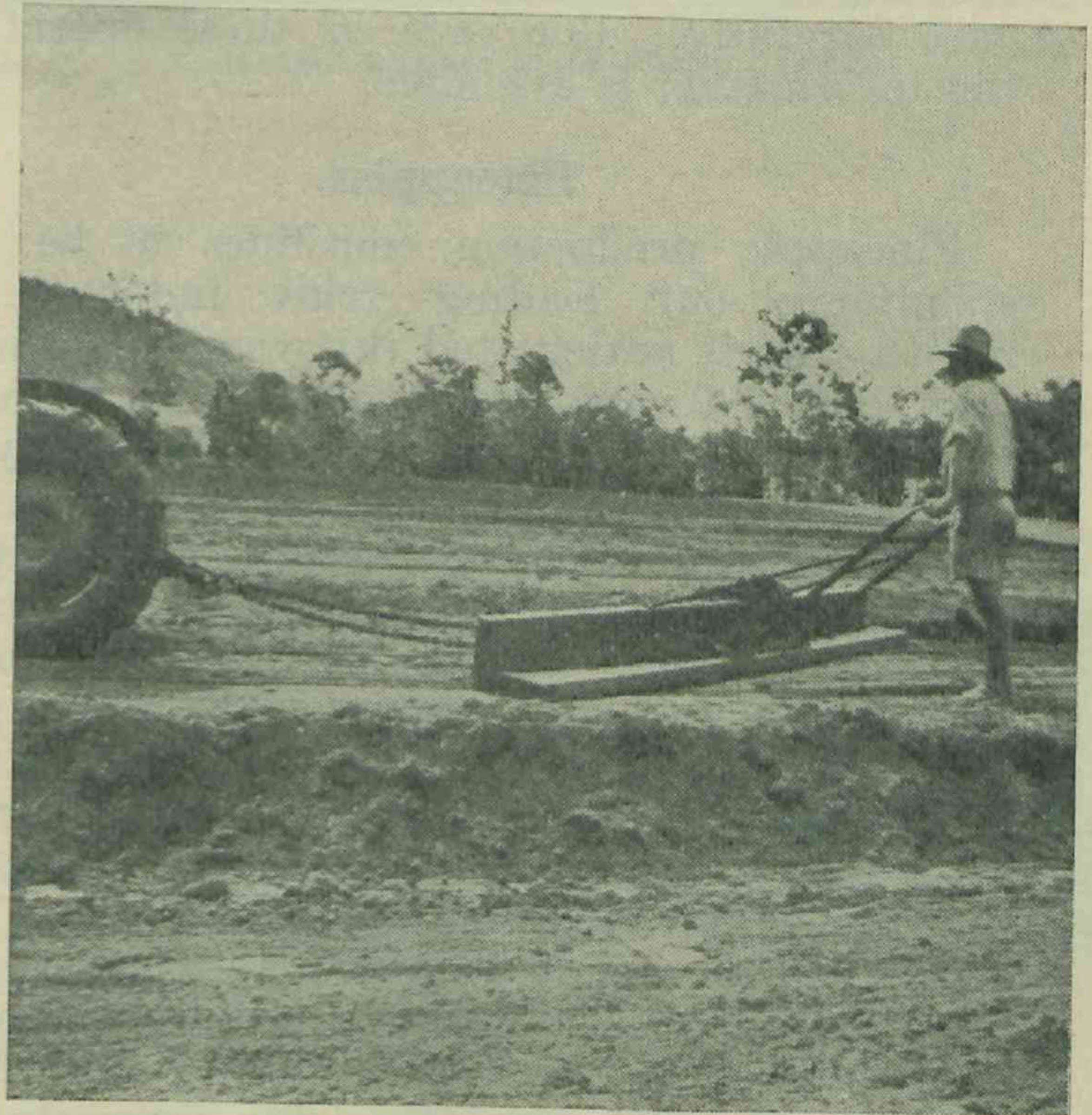
Plate 7.—The Johns Leveller, a Useful Implement for Levelling Land for Irrigation, is Shown Here Moving Soil Across a Bay for Correction of Side Fall.
