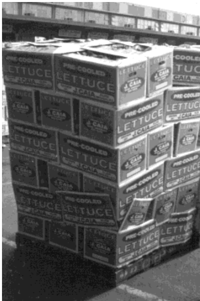
Figure 10. Possible causes of carton collapse: under strength, wet, too high, poorly secured, rough handling.
