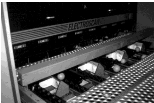
Figure 6. Computer-controlled orange size-grader.
