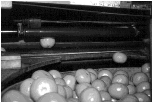
Figure 5. A common belt and roller size-grader for mandarins.
