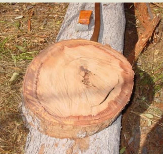
**Figure 4.4** Defect rings caused downgrade to salvage class in this bloodwood log.
