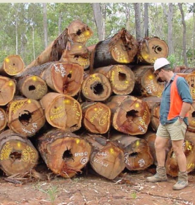
**Figure 4.8** This stack of salvage logs shows pipe defect.
