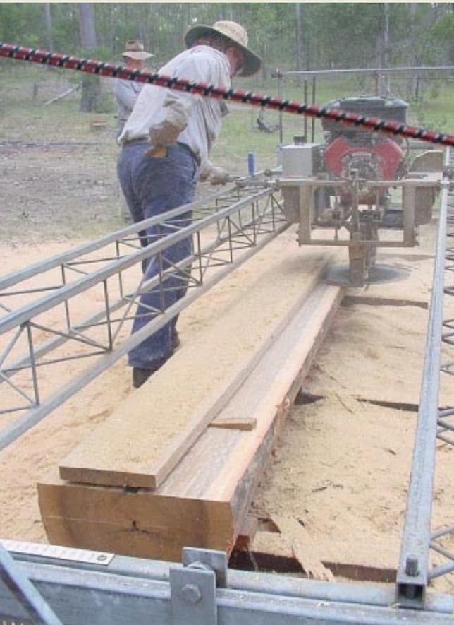
**Figure 3.7** Cutting a 250 mm board required making a 200 mm cut from one side, flipping the saw over and cutting the edge board off the outside of the log and then making the final 50 mm cut.
