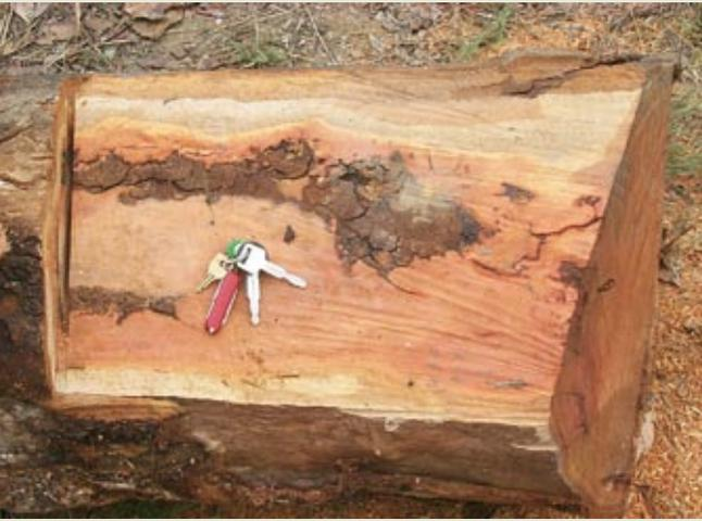
**Figure 1.6** Longicorn beetle damage to grey gum. Insect damage is common in trees stressed from overstocking.
