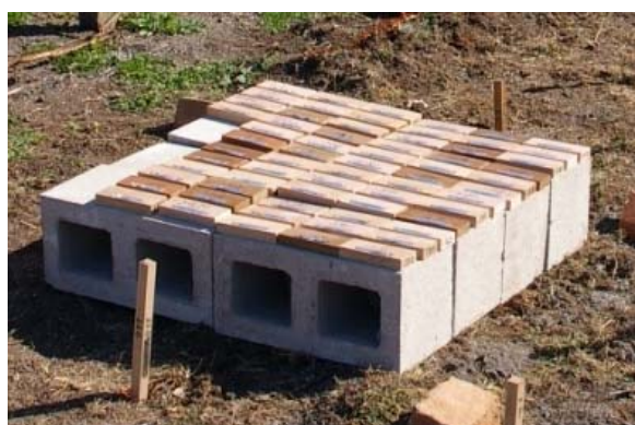
Figure 4 Ground-proximity samples installed at Dalby (shade cloth lid removed for photograph)
